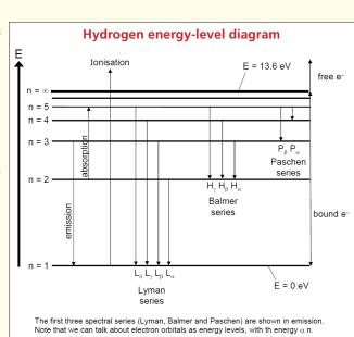
The electronvolt, eV, is a unit of energy,  $1 \text{ eV} = 1.602 \times 10^{-19} \text{ J}$
