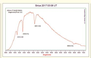
Raw profile of Sirius. The hump in the graph is the result of the star's color and the spectral sensitivity of the camera. The primary hydrogen Balmer lines are labeled.
