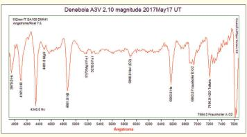
A raw profile of Denebola has been processed through a technique called normalization, which removes the hump and equalizes the spectral intensities. A variety of absorption lines are identified.
