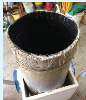
6. Used Elmer's Glue-All for the end of the frayed tube and held it in place with large paperclips.
