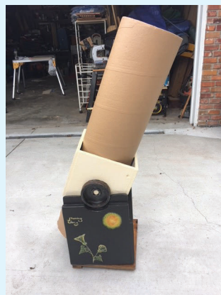
16, 17. You can see that the focuser is on the opposite side of a normal scope's. And there is no spotter scope!
