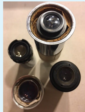
4, 5. All these eyepieces are made with metal pipes, pieces of glass, cardboard, and masking tape.
