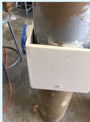
21. Good shot of the original state of the tube with silver paint, sand paint, chipping and peeling, and the mirror cell had no paint on it at all.
