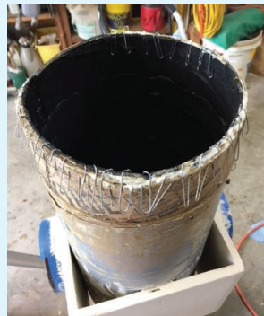
6. Used Elmer's Glue-All for the end of the frayed tube and held it in place with large paperclips.
