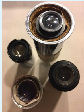
4, 5. All these eyepieces are made with metal pipes, pieces of glass, cardboard, and masking tape.
