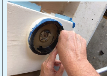
20. The harmonic balancers, a.k.a. altitude bearings, needed the peeling paint removed.
