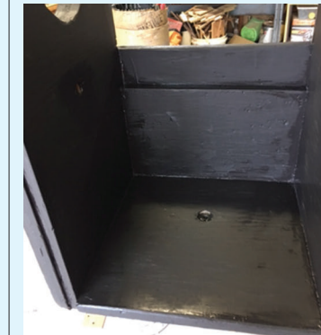
13. The inside of the base needed a rough sanding to knock down some raised grain and paint drip marks.
