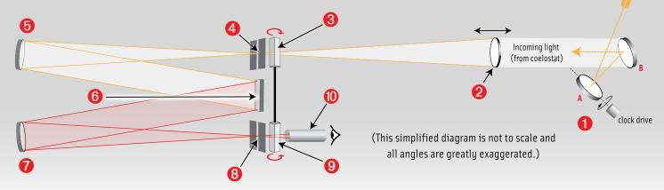
**COELOSTAT** consists of two flat mirrors arranged to direct the Sun's light in a fixed direction. The first (A) is mounted equatorially, and driven by a clock drive to follow the Sun's path. The second (B) is alt-az mounted and adjusted to reflect the beam from the first mirror to the objective lens.
