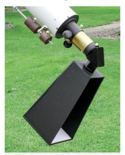
Figure 1. Hossfield Pyramid constructed of black foam board with a Bristol board projection screen. When used in this position, with a star diagonal, the screen is always in the shade, permitting bright, contrasty views of the Sun.
