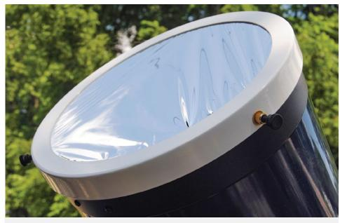
Figure 2. Pre-mounted Baader visual filter attached to a 10-inch Schmidt-Cassegrain telescope; nylon screws hold the filter securely in place.
