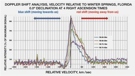
Chart 3: Plot of relative velocity calculated with Microsoft Excel from Doppler shift, using the equation at left. The horizontal axis now shows relative velocitu.
