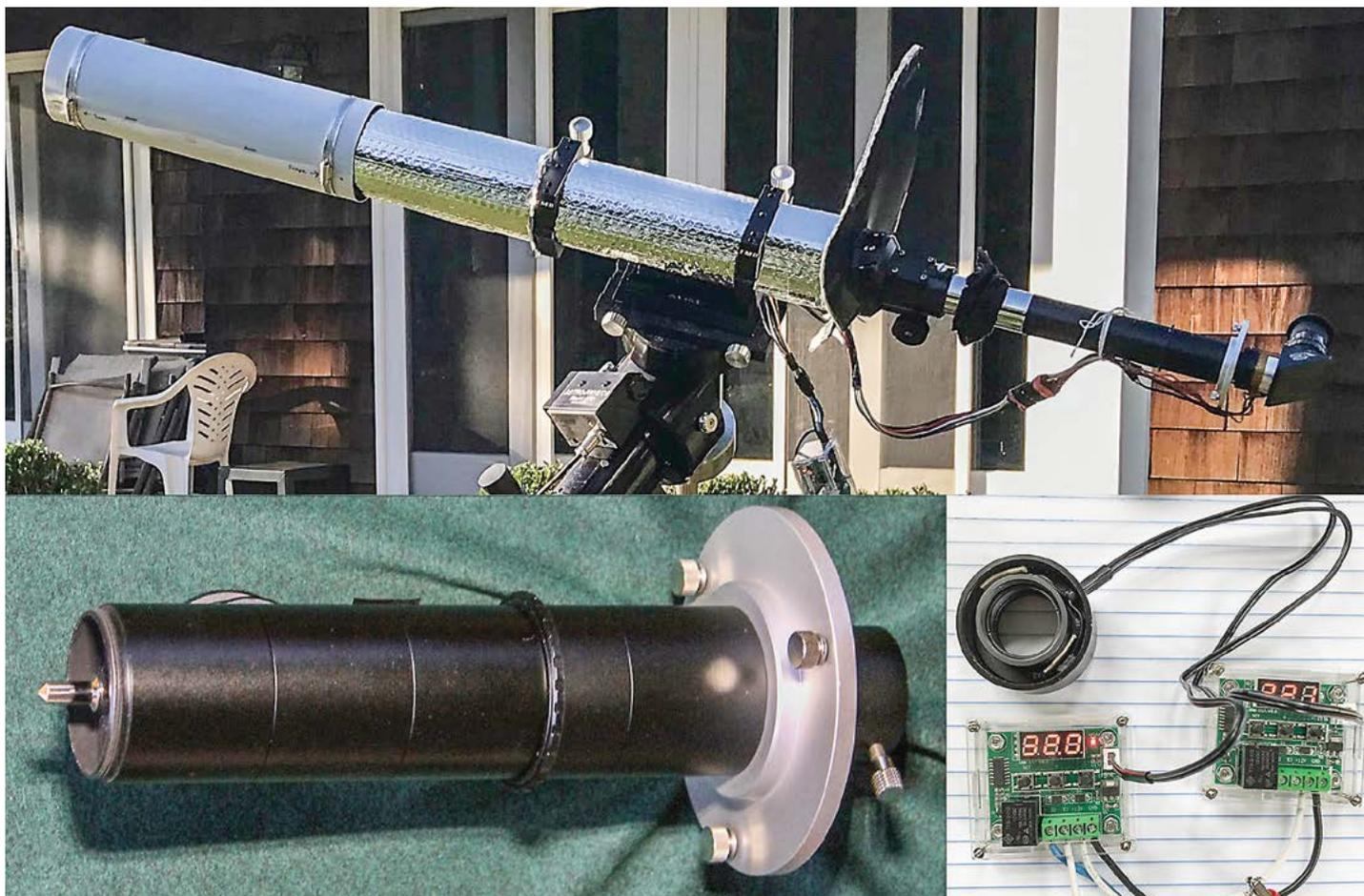
Figure 2: Hripcsak's telescope, the modified Baader prominence viewer with the cone exposed, and the homemade oven for the 530.3 nm filter.
