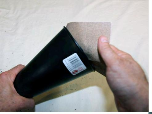
**Step 5.** Using the sandpaper, smooth all the cut surfaces on both ends of the funnel.
