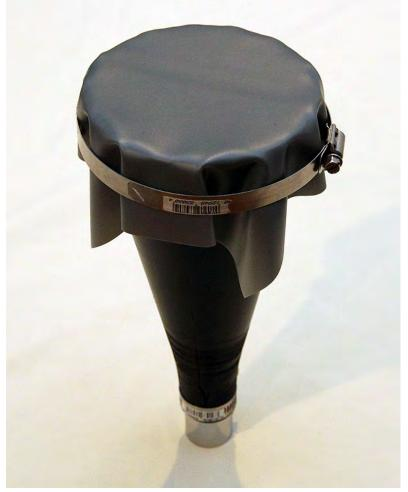
...and, using the screwdriver, tighten it around the funnel to securely hold the screen; as the clamp begins to get purchase on the funnel and screen, gently pull down all around the loose edge of the material so that the screen ends up flat and taut over the funnel's wide opening. This is an iterative process; you'll need to pull down on the material after each turn of the screw to keep it taut.
