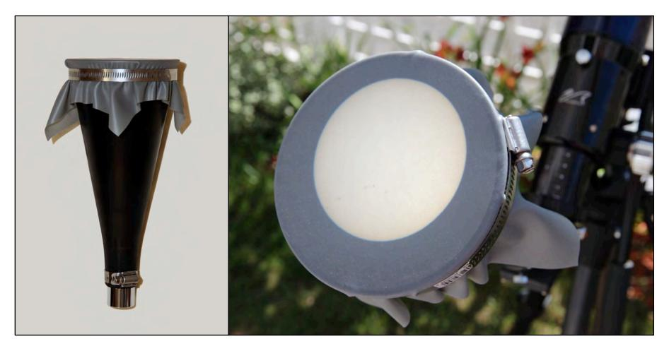
Origin of the Sun Funnel: Amateur astronomers Gene Zajac and Chuck Bueter adapted (<a href="http://bit.ly/1raqocH">http://bit.ly/1raqocH</a>) an existing design for a 2003 Great Lakes Planetarium Association Conference workshop. The rear-screen projection material shown here is an idea borrowed from Bruce Hegerberg's Sun Gun (<a href="http://bit.ly/23SVC5N">http://bit.ly/23SVC5N</a>).
