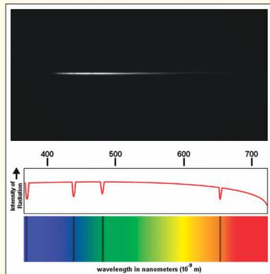
Images above show a typical spectrum from an amateur grating (Star Analyser). Note the absorption lines on the left. The second image shows a plot of intensity vs. wavelength. The "dips" in the graph represent absorption lines, which are seen in the spectrum below as discrete dark lines.
