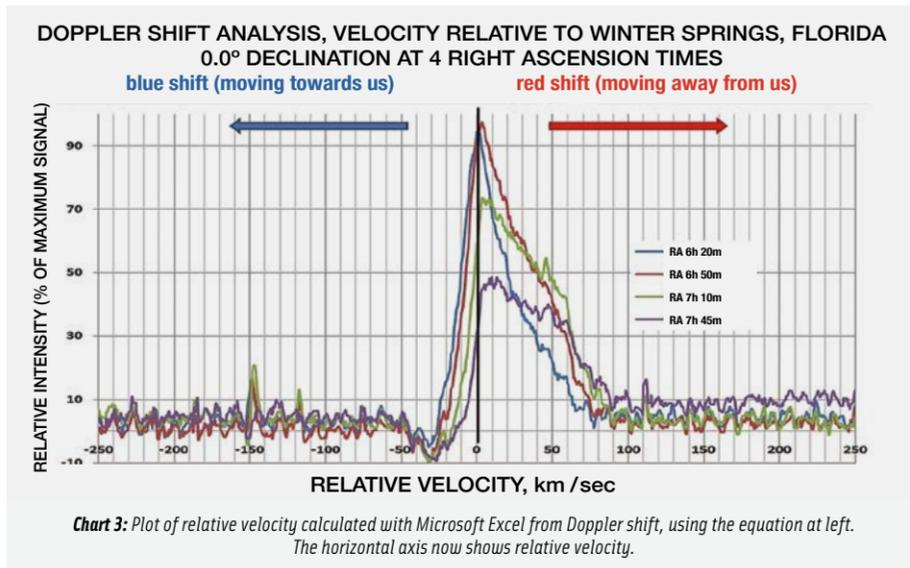
Chart 3: Plot of relative velocity calculated with Microsoft Excel from Doppler shift, using the equation at left. The horizontal axis now shows relative velocity.
