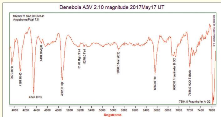
A raw profile of Denebola has been processed through a technique called normalization, which removes the hump and equalizes the spectral intensities. A variety of absorption lines are identified.
