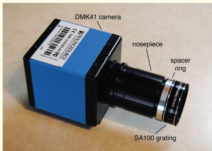
A simple converging beam slitless spectrograph can be created by attaching a screw-in transmission grating in front of a camera.
