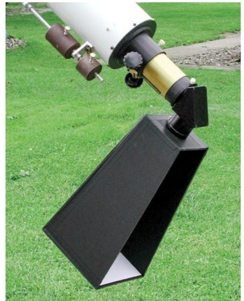
Figure 1. Hossfeld Pyramid constructed of black foam board with a Bristol board projection screen. When used in this position, with a star diagonal, the screen is always in the shade, permitting bright, contrasty views of the Sun.
