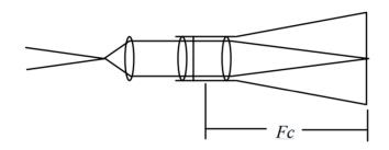
In the Afocal projection system, the telescope and eyepiece are focused on an object and the camera, with its lens in place and focused at infinity, is placed behind the eyepiece. Given the camera lens focal length, Fc, and telescope/eyepiece magnification, M, the system focal length is:
