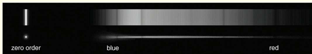
pixel array of the camera, eliminating the introduction of artifacts into the imaged spectrum. Because the grating attaches to the nosepiece of the camera like a standard 1.25-inch eyepiece filter, it is a matter of rotating the grating cell on its threads until it is aligned, then locking it in position. Once aligned, I use a small piece of tape to hold the cell in place.
