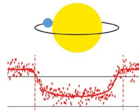
A light curve showing the effects of an exoplanet transiting the face of its host star.
