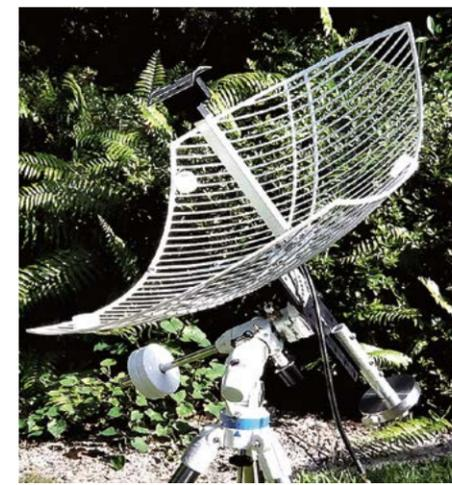
The parabolic reflector mounted on a telescope mount.
