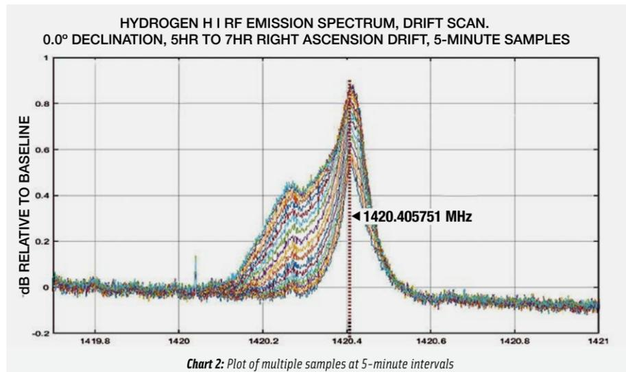
Chart 3 Shows Doppler redshift velocity calculations. In chart 2, you can see a left bias in the data: a significant portion of the data is at frequencies less than 1420.405751 MHz. This lower-frequency content is due to the Doppler shift caused by this area of our galaxy moving away from Earth: a redshift. The frequency shift can be converted to an actual velocity with the following redshift equation
