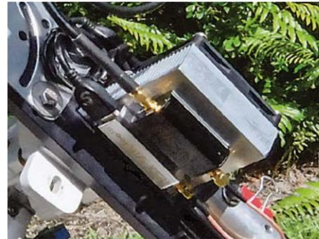
The optional (\$11) but recommended heat sink shown above provides cooling for the SAWbird and SDR and a place to securely mount the components. Keep the connection between the antenna and SAWbird short because cable losses are high at these frequencies.
