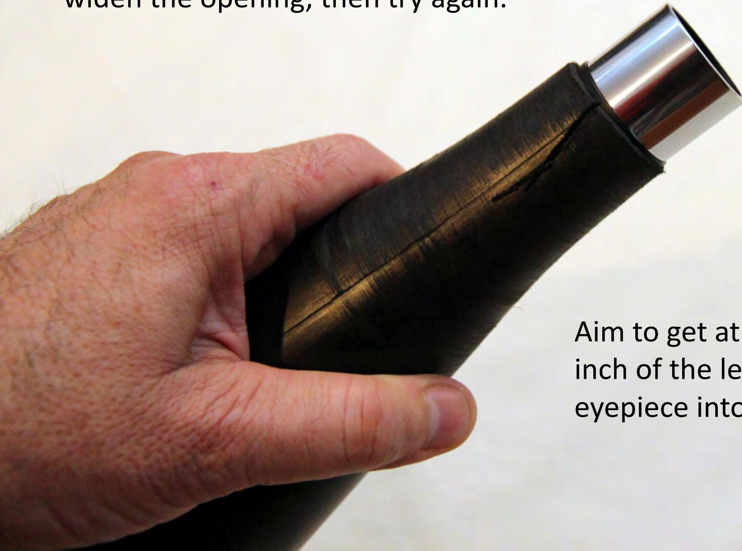
Aim to get at least a half inch of the length of the eyepiece into the funnel.
