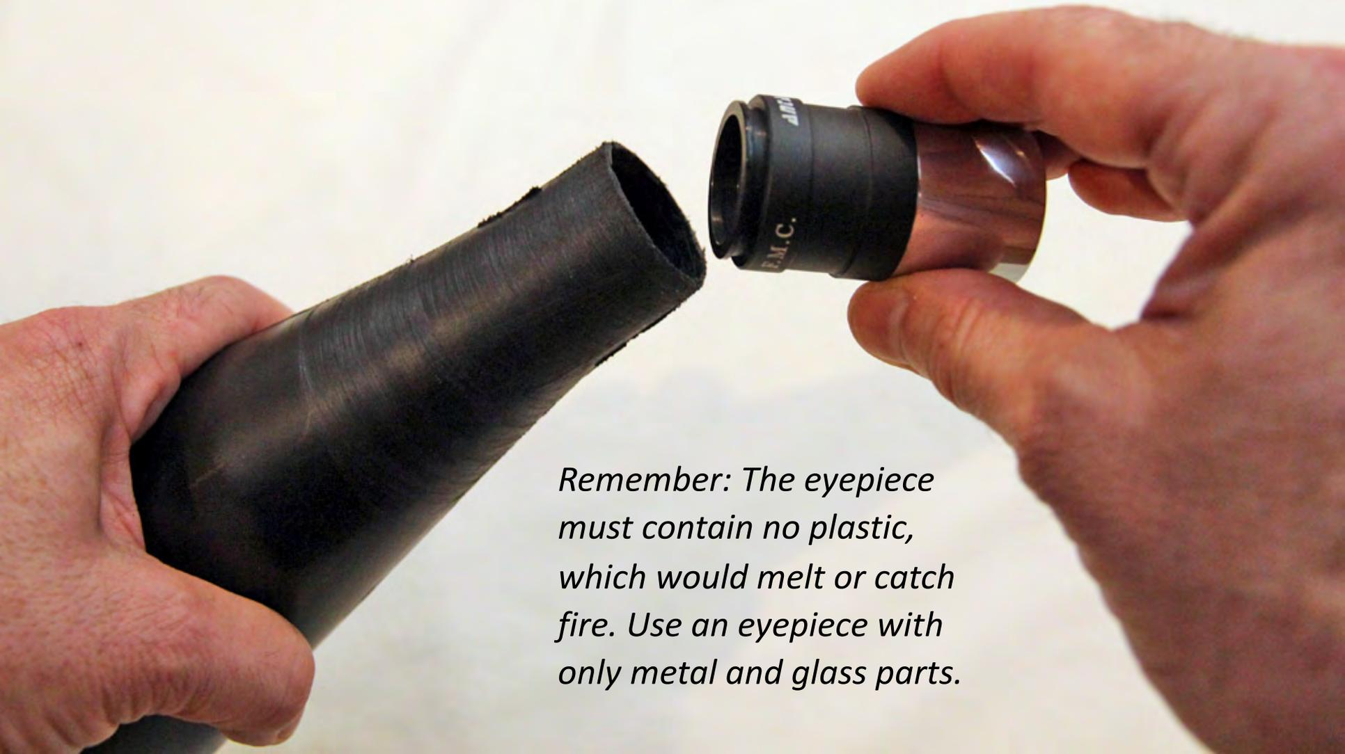
*Remember: The eyepiece must contain no plastic, which would melt or catch fire. Use an eyepiece with only metal and glass parts.*
