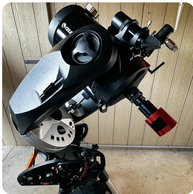
CPC 8" on equatorial wedge configured for imaging with ASIAIR 585MM camera, ASIAIR mini controller, and a Starizona counterweight system. Not shown are cables, filter wheel assembly, camera angle adjuster, and automatic electronic focuser.
